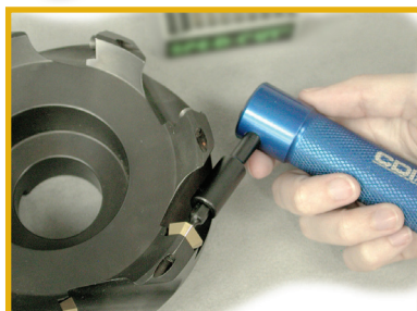
Prevents premature wear of carbide inserts and damage to cutter head due to improper clamp load.
