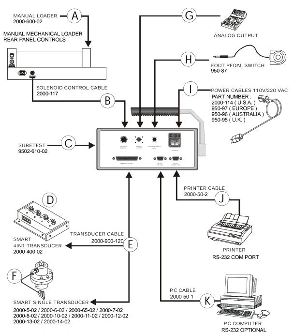
Figure 3-1: SURETEST Torque Tester/Calibrator/Loader Setup
