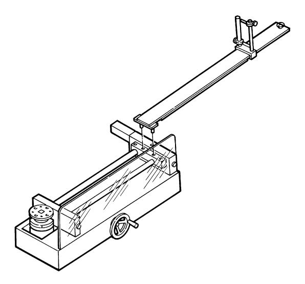
Figure 6-6: 2000-600-02 Manual Loader Extension Arm
