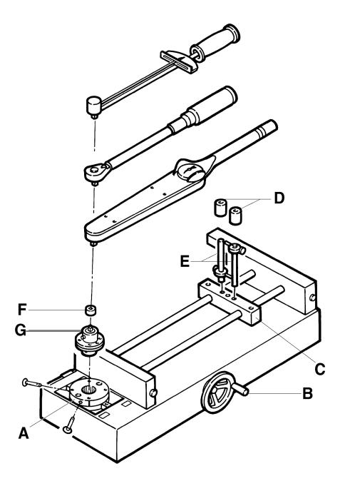
Figure 6-2: 2000-600-02 Manual Loader, Exploded View
