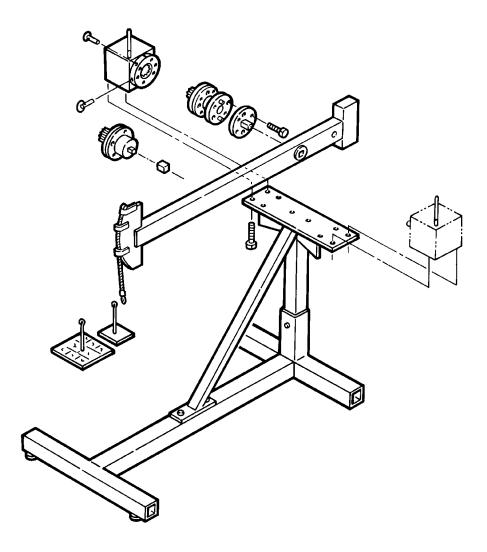
Figure 5-2: Single High Torque Transducer Mounting Detail
