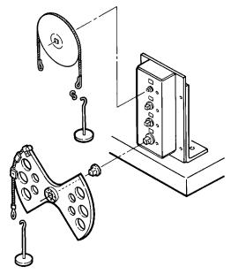
Figure 5-3: 4-in-1 Transducer Mounting Detail
