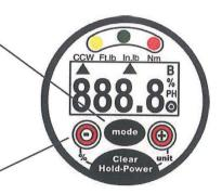
2. Then press and hold the Target - button, (wait for the contrast to change)
